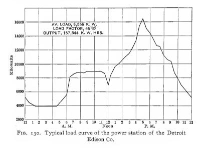
Fig. 130 has been selected as a characteristic lighting curve in a large station. It shows two characteristic peaks, the main one naturally occurring in the evening. Between the peak hours there are certain parts of the day during which very little light is used, but the power load which always accompanies a lighting load tends to fill up the depressions.
